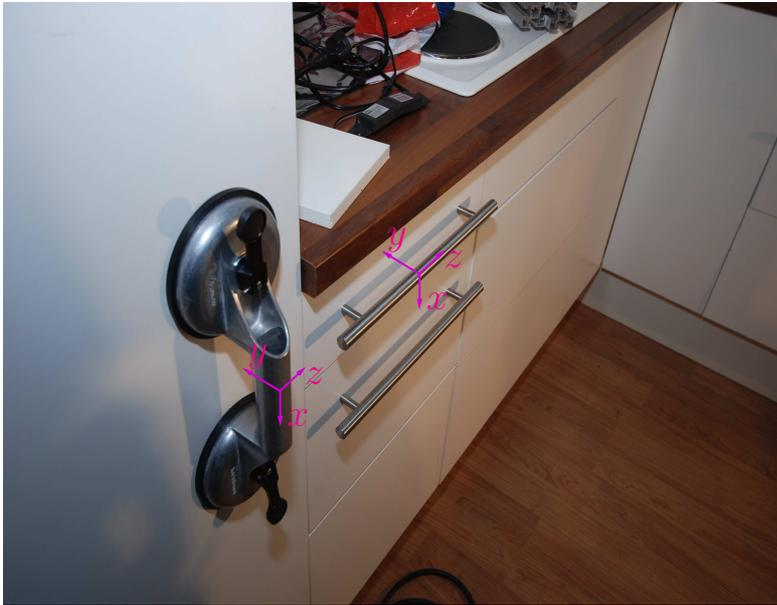
FIGURE 5.4. Experimental setup. The base coordinate system is plotted on two potential contact points to visualize the true direction of motion if the robot stands right in front of the devices.
