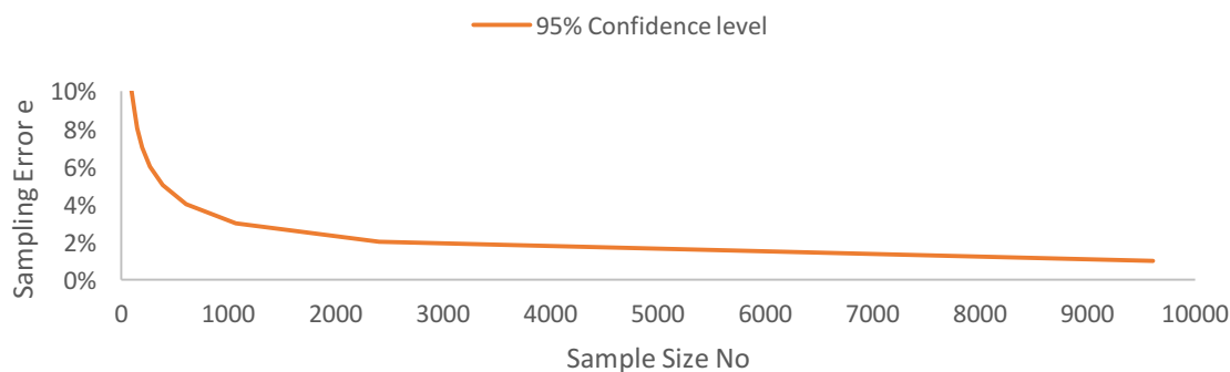
Figure 4.2 Dependence of sampling error on sample size with a margin of sampling error calculated for infinite populations. Source: Own elaboration based on (Puszczak et al., 2013)
