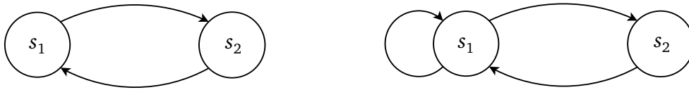
Figure 2.5: Periodic (left) and aperiodic (right) Markov chains with state space \{s_1, s_2\} .
