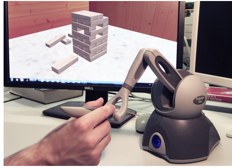
Figure 2.1: A kinesthetic haptic device (Geomagic Touch [79]) to interact with a virtual environment.
