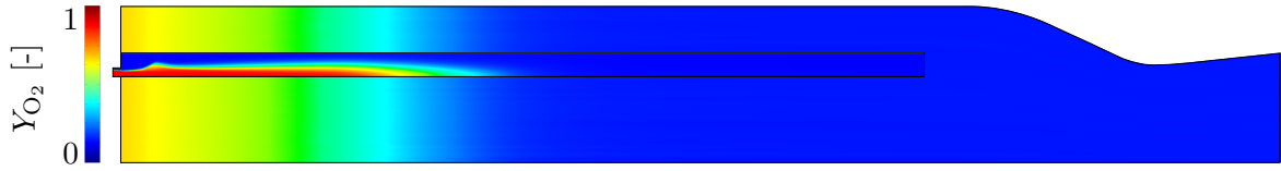
Fig. 6.8.: O_2 mass fraction of the mean flow for the acoustic simulation together with its detailed distribution in the single flame case.
