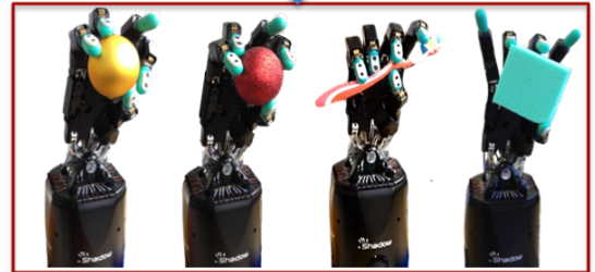
Fig. 1. The Shadow Dexterous Hand with BioTac Tactile Sensor-Employing the proposed tactile transfer learning method enables the Shadow Hand to re-use its prior knowledge when discriminating new objects while having very few tactile data samples.
