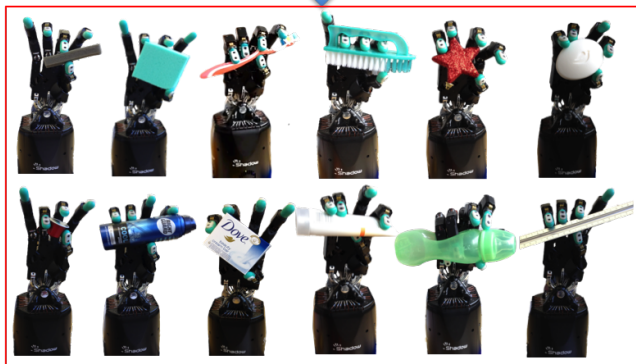
Fig. 1. The Shadow Hand with BioTac robotic skin. Employing the proposed tactile transfer learning method the Shadow Hand could re-use its prior knowledge while discriminating new objects from their texture with a very few trials. The illustrated formula is the regularizer term of the adapted LS-SVM in (2). The weight assigned to each prior knowledge \lambda was found by minimizing Eq.(2). K is the number of prior knowledge.
