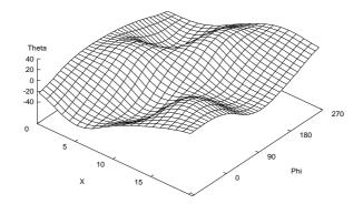
Figure 16: Solution of the "truck backer-upper" problem: output  $\theta$  after learning ( $\theta$  was initialised as zero for all inputs).
