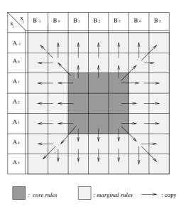
Figure 3: The outputs of the marginal rules are copied from that of the neighbouring core rules.
