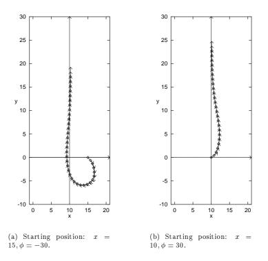
Figure 17: Two motion trajectories produced by the trained fuzzy controller.
