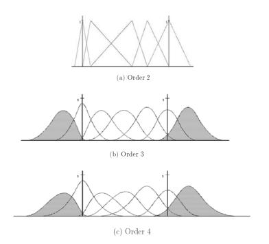
Figure 2: Non-uniform B-functions of different orders defined for real and virtual linguistic terms by the same knot vector (virtual linguistic terms: shaded).
