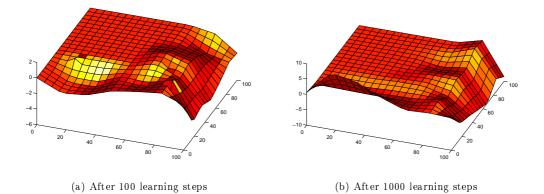
Figure 21: The control surfaces for contour tracking.
