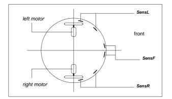
Figure 18: Sensors and motors of the Khepera robot.
