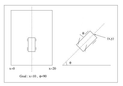
Figure 15: The start and goal position of the truck.
