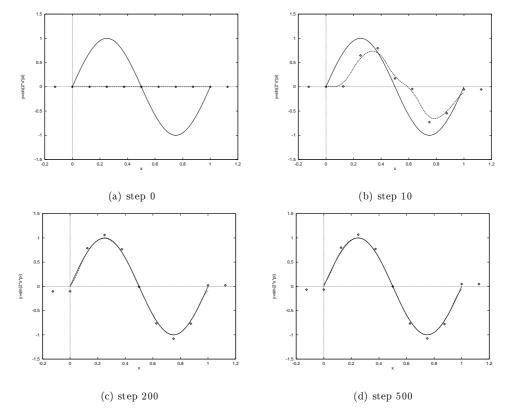
Figure 9: Optimisation of positions of the fuzzy singletons defined on the output ( $\epsilon = 1$ ).
