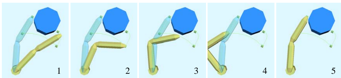
Figure 4.4: A sequence of configurations along the planned motion for the 2-DOF manipulator.
