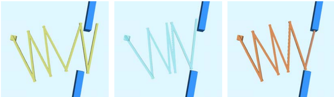
Figure 4.14: Failure of local planning for an 8-DOF planar manipulator. If it is attempted to move link 8 approximately parallel through an opening (left and center), every alternative path will either push link 8 further in collision or link 7 collides with the obstacle, thus no solution can be found. The configuration of worst rating is shown in the right image.
