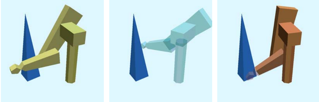
Figure 4.13: Failure of local planning for a 6-DOF manipulator. The task is to move from one side of an obstacle to the other side (left and center). The highest rating increase is achieved by moving downwards, i.e. turning link 2. This reaches its lower limit, and link 3 cannot be turned up again, as this would decrease the rating (right).
