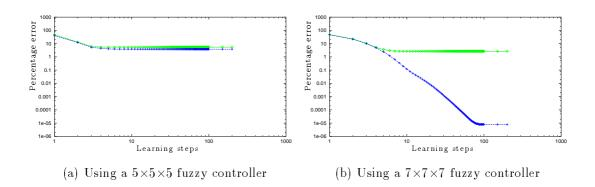
Figure 3: The error curves of two fuzzy controllers with different partition granularity.
