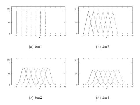
Figure 1: Fuzzy sets defined by B-spline basis functions of different orders.
