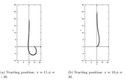
Fig. 13. Two motion trajectories produced by the trained fuzzy controller of the "truck backer-upper" problem.
