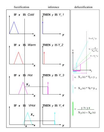
**Fig. 5.** A SISO system with B-functions of order 2  $(X_i(x))$ : firing strength of rule i;  $y_i$ : the contribution of rule i to the output).
