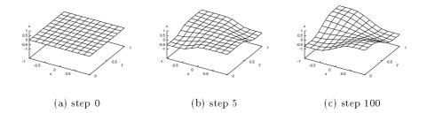
**Fig. 10.** The control surfaces during the optimisation for approximating the function  $z = sin(2\pi x) \cdot cos(\pi y)$ , with  $-1 \le x \le 1$  and  $0 \le y \le 1$ . The membership functions defining the real and virtual linguistic terms of x and y are 7 B-functions of order 3 for both x and y.
