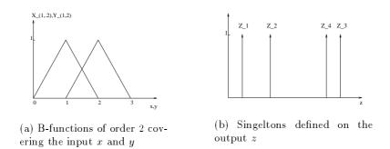
Fig. 6. Linguistic terms used in a Two-Input-One-Output system
