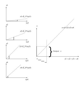
Fig. 8. Defuzzification by blending the control vertices with B-function values
