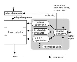
Fig. 1. Integration of subgoal planning and sensor-based plan execution.
