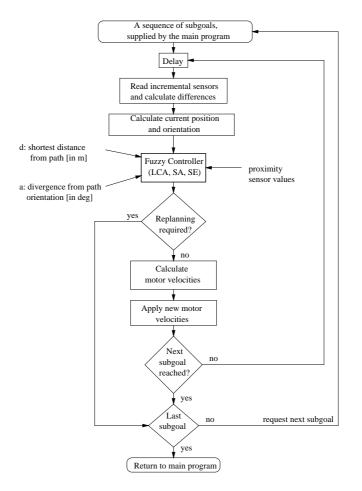
Fig. 10. Flow chart for integrating "subgoal planning" and "local collision avoidance".
