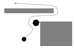
Fig. 13. Subgoal approaching with an unknown obstacle.
