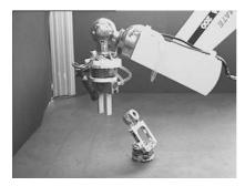
Fig. 2. In order to hand over an object to a manipulator, the mobile robot must receive coordinating commands from other robots or the central supervision system.
