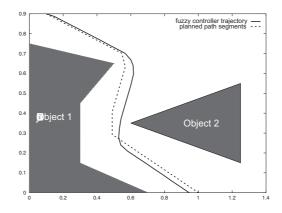
Fig. 8. Trajectory of the controller using the rule base "subgoal approach".
