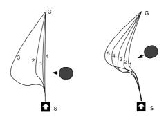
Fig. 14. Collision-avoidance with a dynamic obstacle.
