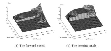
Fig. 3. Mapping sensor data to the control output.
