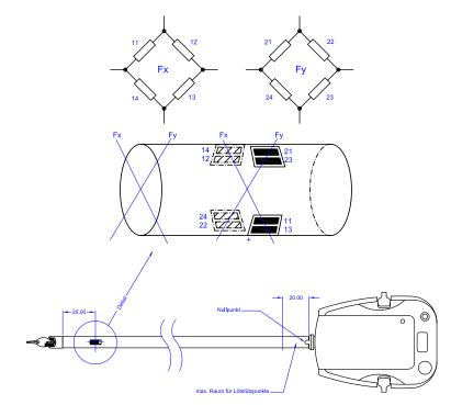
${\bf Fig. \ 3. \ Strain \ gauge \ application \ blueprint}$
