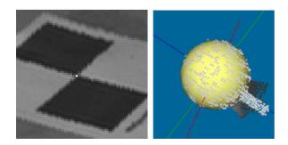
figure 7: The Z+F software provides a method for finding two different types of predefined targets: *Left*: The "chess pattern" Target [2], *Right*: The "Bowl" Target
