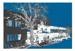
**figure 8**: The figure shows a 3D point cloud of several scans of high density like they can be visualised by using LFM Server
