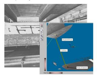
**figure 9:** The figure shows the reflectance image of a highway bridge and a simple "on the job" measurement: The user can control the distance of a selected spot on the road to the bridge directly after the scan just by marking it in the reflectance image.
