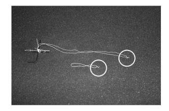
Figure 3: Ruptured suture. All sutures ruptured at the knot.
