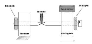
Figure 2: experimental setup with the fixed GORE-TEX<sup>®</sup> Suture between the two robot arms.
