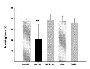
Figure 6: Breaking forces of the pean, clip and control group of both experiments (mean  $\pm$  standard deviation). kp = knot-pusher; \*\* significantly decreased p < 0.01
