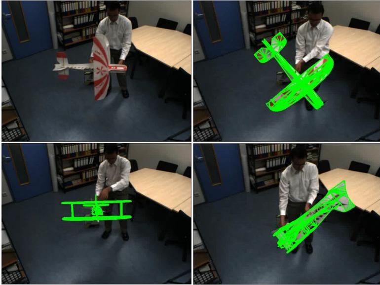
Figure 6: Tracking of a model aircraft with fused CCD and Edges likelihood based on a real video sequence. Critical poses for tracking (bottom row).
