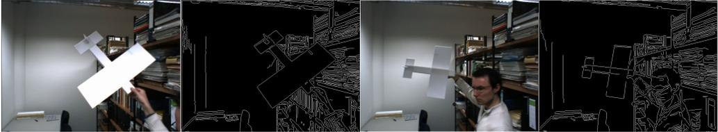
Figure 1: Local color statistics efficiently deal with situations showing a significant difference between foreground and background color regions (left frame), but may fail when a weak separation is present (right frame). On the contrary, an intensity-based tracker works well when luminance edges can be reliably detected (right edge map), but may be challenged by a locally cluttered background (left edge map).
