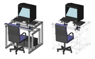
Fig. 2. Master console with PHANToM devices and 3D screen
