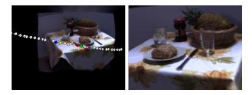
Fig. 8. (Left): A virtual image which shows apart from the scene some of the reference cameras which are depicted by a part of their viewing frusta. The colored reference cameras are chosen by the view selection algorithm and contribute to rendering this virtual image. (Right): A close-up virtual view onto the objects of interest.
