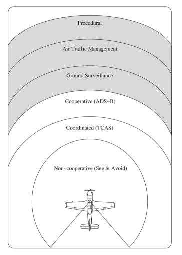
Fig. 8. Collision avoidance mechanisms available to civil aviation. In gray are the techniques to ensure separation. Adapted from [54].
