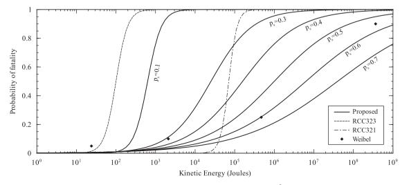
**Fig. 5.** The probability of fatality as a function of kinetic energy impact for the proposed model with  $\alpha = 10^6$  J,  $\beta = 100$  J and for several values of  $p_s$ . For comparison purposes the estimates of Weibel [49] as well as the models of RCC321 [51] and RCC323 [47] are given.
