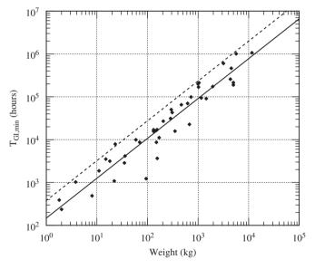
**Fig. 7.** The calculated  $T_{\rm GI}$  requirement versus the corresponding MTOW for 43 UAS of different types and sizes. The calculations are done for a population density of 200 people per km<sup>2</sup>,  $\alpha = 10^6$ ,  $\beta = 10^2$  and  $p_{\rm s} = 0.5$ . The relationship is approximately linear with respect to their logarithms. The dotted line corresponds to the requirement derived with a 300% safety margin added.
