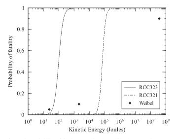
Fig. 4. The probability of fatality as a function of kinetic energy impact as estimated by Weibel [49] and models derived in RCC321 [51] and RCC323 [47].
