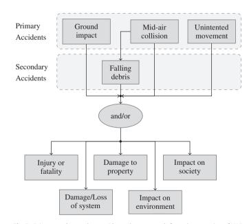
Fig. 3. Primary and secondary accidents that can result from the operation of UAS.
