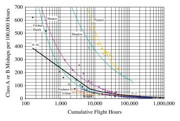
Fig. 9. Comparison of lifetime class. A mishaps of the F-16 military aircraft and various military UAS (1986–2006) [64].
