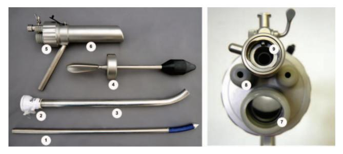
Figure 3. The new set of instruments (ISSA) designed to permit sterile sigmoid access for transcolonic surgery; (1) part flexible obturator, (2) trocar head, (3) trocar tube, (4) TEM obturator, (5) modified TEM cap, (6) modified rectoscope, (7) trocar port, (8) instrument ports, and (9) optical port.
