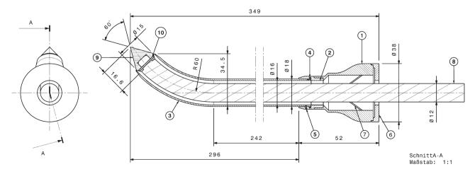
Figure 1. Cross-section of the ISSA trocar with inserted part flexible obturator; (1) trocar head, (2) trocar adapter, (3) trocar tube, (4) Oring seal, (5) bayonet mechanism, (6) front cap, (7) trocar valve, (8) part flexible obturator, (9) conic front end, and (10) pin.
