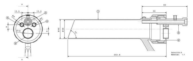
Figure 2. Cross-section of the modified TEM device; (1) rectoscope, (2) TEM cap, (3) shortened optic port, (4) instrument ports, and (5) trocar port.
