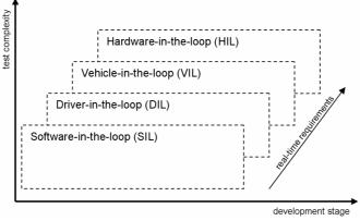
Figure 1: Development stages vs. test tools
