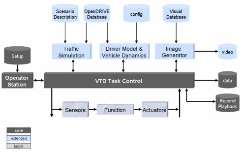
Figure 5: The categories of VTD components
