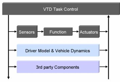
Figure 4: Harmonized I/O between VTD and other components
