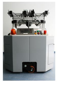
Figure 4.8: Rear view of the F5 robot with the control panel, the touchpad and the warning light.
