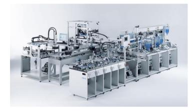
Figure 2.6: Changeable Factory consisting of several Festo Modular Production System workstations. Photograph: Festo Didactic.
