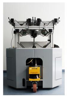
Figure 4.6: Front view of the F5 robot. Noteworthy is the 180  $^\circ$  Leuze laser range finder.
