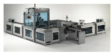
Figure 6.11: Changeable Factory made of Festo MPS modules. Photograph: Festo Didactic.
