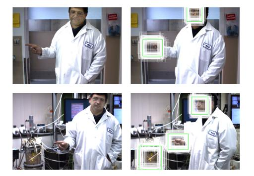
Figure 6.10: In the shown pictures, the scientist's face and hand (upper row) are detected and tracked by the robot until he arrives at a fermentor station (lower row) where the fermentor is detected as well. This way and in combination with the automated mapping and path planning a human guide can teach a lab walkthrough and indicate positions of interest for a repetitive fermentor monitoring routine, without preprogramming any knowledge about the environment.
