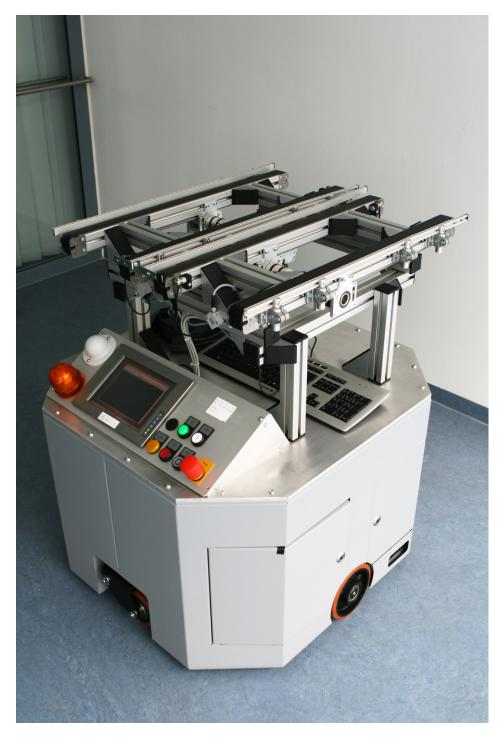
Figure 4.10: The F5 robot with the control panel and touchpad on the rear side and two pairs of conveyor belts mounted on top of the platform to pick up and hand over standardised Schaefer boxes. Light barriers at the entry points of the conveyor belt indicate their occupation.
