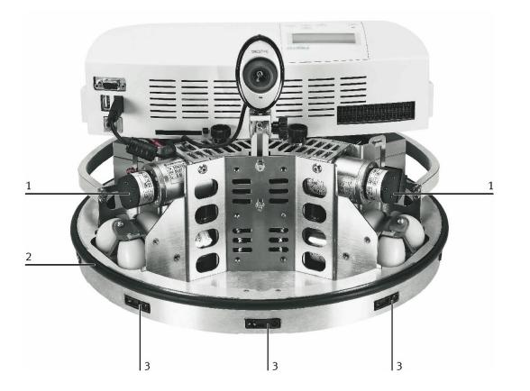
Incremental encoder (1) Impact strip, anti-collision sensor (2) Distance measuring sensors (3)
