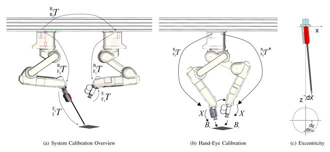
Figure 3. **System Calibration.** Figure 3(a) depicts a schematic overview of the kinematic chain. The hand-eye calibration is exemplified in illustration 3(b). Figure 3(c) shows excentricity and play of the instrument shaft.
