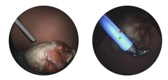
Figure 12. Left image: Initial estimation of the instrument pose, derived from sensor readings. Right image: Mismatch of the model scaling factor and the instrument due to strong specular reflections.
