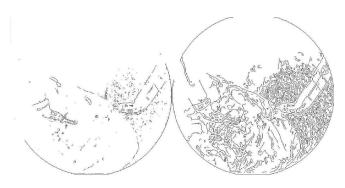
Figure 7. **Edge detection.** The images show edge detection results of the Sobel (left) and the Canny (right) filter. In both cases the tool shaft can hardly be distinguished from background noise. The organ surface comprises many small vessels and structures that raise edges in the vicinity of the tool tip.
