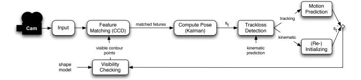
Figure 5. Tracking Pipeline. The camera pose can be obtained after calibrating the extrinsic parameters and the overall system. The kinematic measurement of the instrument in 6 degrees of freedom is transfered to a 2D model with 4 DoF  $(t_x, t_y, h, \theta_x)$ . It is used to (re-)initialize the Contracting Curve Density algorithm and to supervise the tracking quality.
