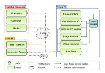
Figure 2. **Software Architecture.** The software of the system is distributed across 3 PC's that communicate via network connections
