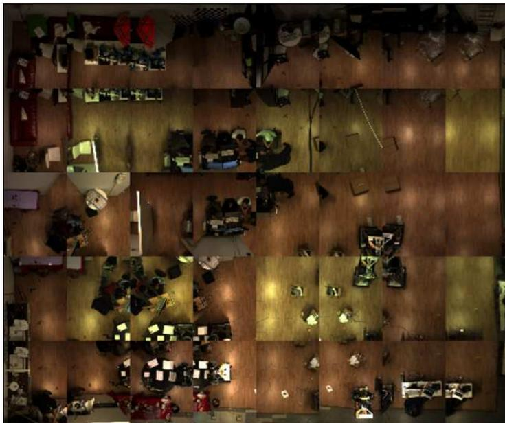
Figure 9: Tiled joint view of the 40 cameras observing the apartment mockup. Different illumination conditions are caused by object shadows, while variant chromatic appearances are caused by using different camera models. Specular reflections result from light sources above the ceiling-mounted cameras.
