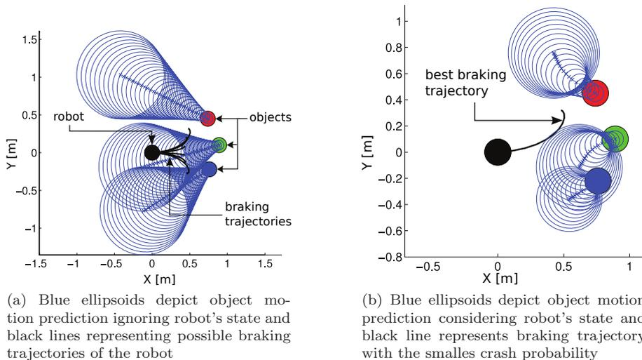
Figure 15: Difference between active and passive workspace objects.
