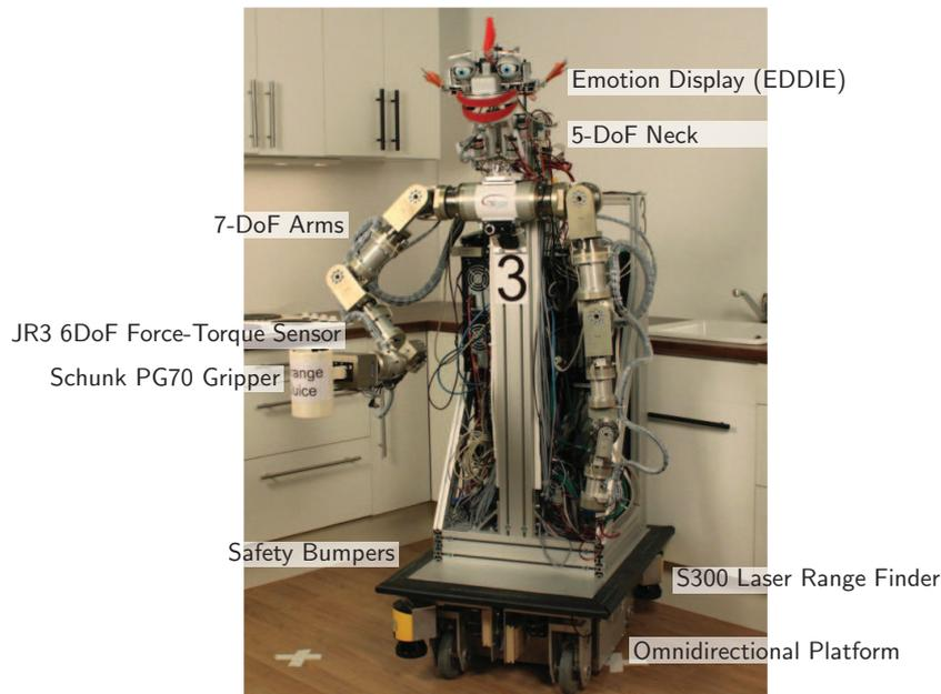
Figure 3: Robot hardware overview.
