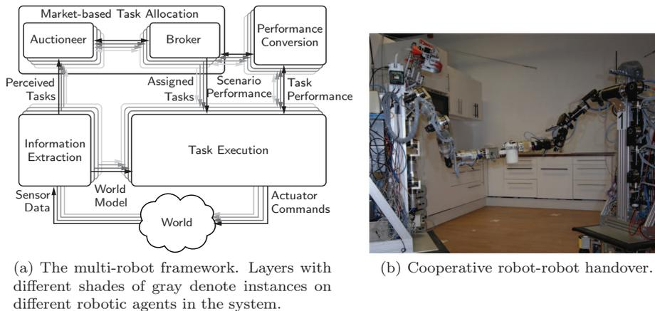
Figure 13: The multi-robot framework and an application example.
