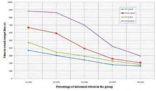
Figure 5. Time taken for the flock center to reach the right-most quarter of the arena's length vs.different proportions of informed robots.
