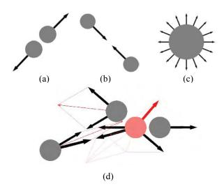
Figure 3. Potential field vectors for flock formation, (a) Separation vector, (b) Cohesion vector, (c) A random vector representing movement of the robots in a random direction, (d) Calculation of resultant vector, shown by light red vectors. The heavy red vector depicts the direction of target used by informed robots (specified by a red circle).
