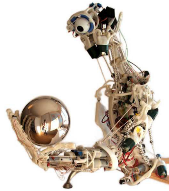
Fig. 1. Prototype of the anthropomorphic [10] robot ECCE-I [11] developed within the EU-funded project ECCEROBOT [12]. The skeleton is hand-crafted using polymorph—a caprolactone polymer—which can easily be molded. The human muscles are imitated by elastic, tendon-driven actuators comprising a DC motor and gearbox in series with a kite line and shock cord as tendon.
