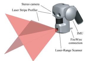
Fig. 1. The DLR 3D-Modeler and its components.
