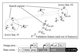
Fig. 5. Top: Pictorial schematic on the 2-D estimations involved. Two *active* features p and q as well as the resulting estimation steps on a further feature v are detailed. The latter is tracked using the regular KLT feature tracker. Bottom: Time evolution of state estimation w.r.t. the image processing steps.
