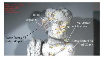
Fig. 6. Detail of a frame including two *active* features, three validation features, and a number of current and past regular features.
