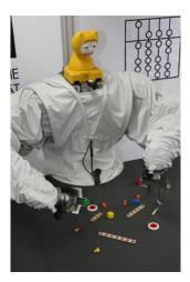
Fig. 1. Human-robot interaction system. The robot has a pair of manipulator arms with grippers, mounted in position to resemble human arms, and an animatronic talking head [10] capable of producing facial expressions, rigid head motion, and lip-synchronised synthesised speech.
