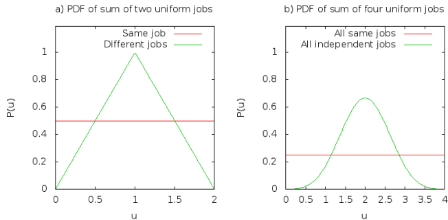
Figure 2: The probability distribution functions of the sum of uniform random variables: a) two jobs and b) four jobs. When combining different jobs (green curve) it is more probable that the combined resource use is centered around the average. In comparison, combining the same jobs (red curve) will have a greater probability of generating a lower or higher combined resource use.
