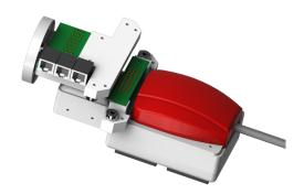
Fig. 3. **Hot-plug instrument** with drive box (red). All necessary electrical connections are established with spring contacts (golden pins on green circuit board). An integrated potentiometer allows a unique tool identification.
