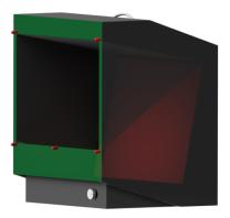
Fig. 2. **Stereo Display.** The five attached infrared LED's (red dots) form a plane (green) that needs to be calibrated to the actual view plane of the monitor (red). The stereo image is generated by fusing two images via a semi-transparent mirror.
