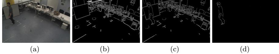
**Fig. 4.** Edge-based background subtraction. (a) Original frame. (b) Learned background model. (c) Unsegmented foreground edge. (d) Segmented foreground edge.
