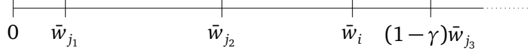
Figure 5.4: Illustration of steady state conic combination (SSCC): \bar{w}_i \in C(\bar{w}_{j_1}, \dots, \bar{w}_{j_l}) can be larger than some \bar{w}_j but is bounded by at least one \bar{w}_j with j \in \{j_1, \dots, j_l\} .
