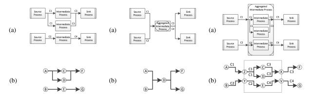
Figure 9: Abstract energy system in (a) USES (b) graph representation, fully disaggregated. Figure 10: Abstract energy system in (a) USES (b) graph representation, fully aggregated. Figure 11: Abstract energy system in (a) USES (b) graph representation, aggregated and disaggregated.
