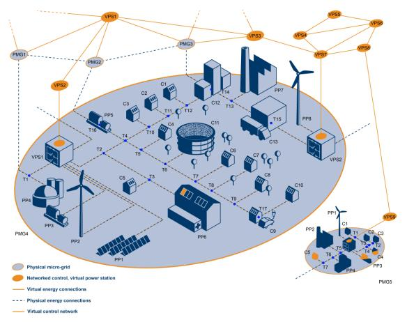
Figure 13: Schematic cut-out of a micro-grid of a distributed energy supply architecture. Source: Based on [GeBr12].
