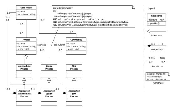
Figure 12: Meta model of USES in the class diagram language of the UML.
