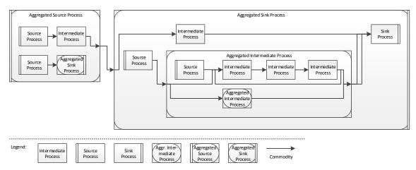
Figure 2: Abstract energy system showing the relationships between all of the defining elements of USES including their sub-elements by taking advantage of the default graphical USES representation.
