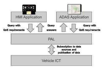
Fig. 3. PAL builds upon the vehicle ICT architecture and provides an interface to the application space.
