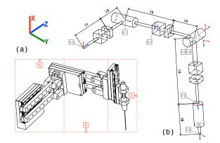
Fig. 3. (a) Serial robot: A and B are parallel coupled joint elements. C is the tool gripper consisting of a prismatic actuator and an optional tool rotator, (b) relevant and simplified model of the serial robot
