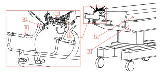
Fig. 4. Ophthalmic operation room; 1: patient, 2: operation table, 3: robot, 4: mounting goggle, 5: goggle arms, 6: robot slider
