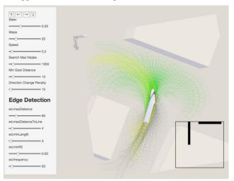
Figure 6. Parking assistance application in the configuration mode.
