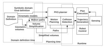
Fig. 2. Overview of the implemented KVP software architecture [1].
