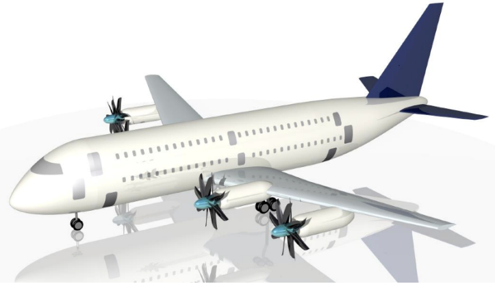
Figure 1. Visualization of the investigated high-capacity turboprop aircraft concept Propcraft P-420. 4
