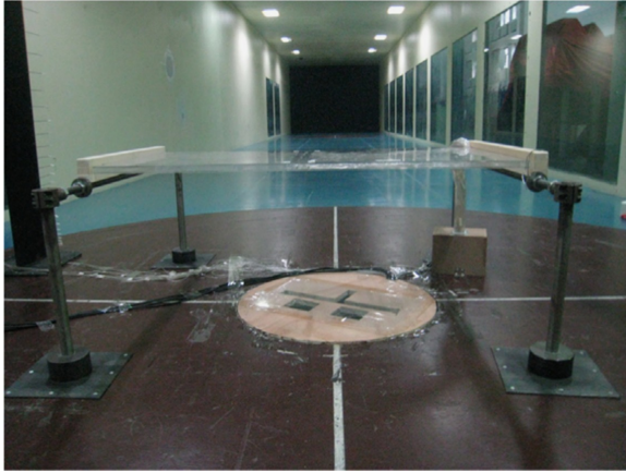
Figure 6.3: Experiment setup of the glass plate in the wind tunnel (photographed from [27]).
