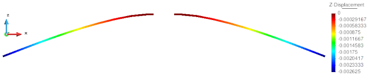
Figure 6.23: Deformation of the blades under gravity load. The deformation is scaled up with a factor of 500.
