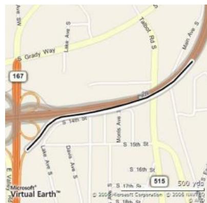
Figure 2.4 Failure cases of finding nearest roads for map matching in crossover, spur/spaghetti intersections, parallel roads, bypass (Krumm et al., 2007). Black thin lines indicate trajectory of GPS observations, white thick roads are correct matching results obtained from Krumm's method, and grey thick roads are results of finding nearest roads.
