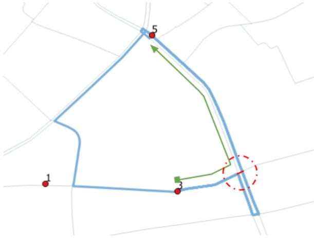
Figure 4.8. An example of missing values. Because of the missing road (red link in the red circle), the actual path (indicated by the green arrow) chosen by car cannot be covered by all the path states (blue lines) between 3<sup>rd</sup> node and 5<sup>th</sup> node.
