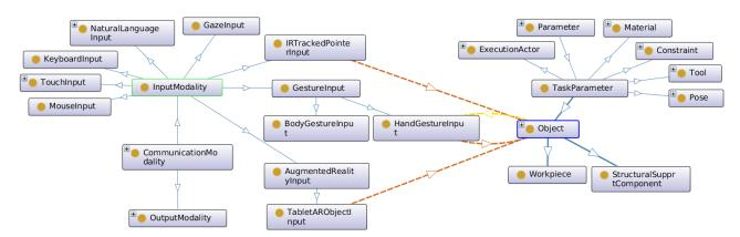
Fig. 3: Taxonomy of input modalities and task parameter types (blue arrows represent subclass relations). This excerpt shows that the input modalities *IRTrackedPointInput*, *HandGestureInput* and *TabletARObjectInput* provide values of parameter type *Object* (orange dashed arrows). The *preferredModality* (yellow dashed arrow) for this parameter type is set to be *HandGestureInput*.
