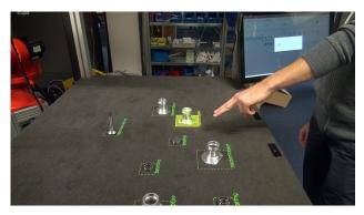
Fig. 6: Detected and highlighted objects on the tabletop. The human operator selects an object by pointing to it. The selected object is highlighted on the tabletop and the GUI
