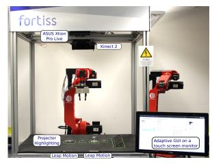
Fig. 1: Cognitive robotic workcell with intuitive graphical user interface integrating further input and output modalities
