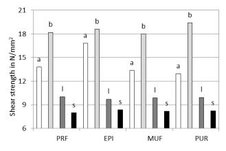
Figure 6: Mean shear strength of the test specimens without further conditioning (a-ash; b-beech; l-larch; s-spruce)
