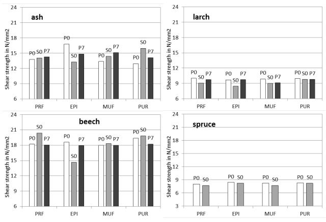
*Figure 8:* Mean shear strength of the test specimens produced with different timber species (P0-planned, fresh; S0-sanded, fresh; P0-planned, 7 days of storage)
