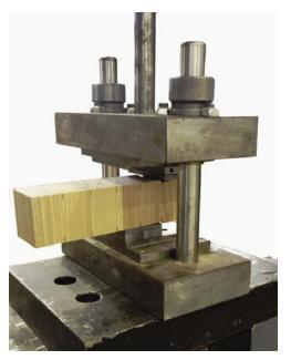
Figure 2: Device for the block shear test
