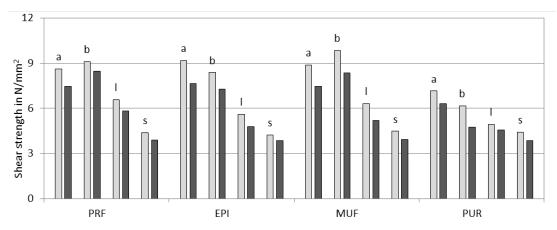
*Figure 7:* Mean shear strength of the test specimens after treatment A2 (light grey bars) and A4 (dark grey bars) (a-ash; b-beech; I-larch; s-spruce)
