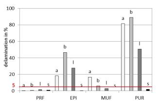
**Figure 4:** Mean delamination of the test specimens produced with different adhesives (a-ash; b-beech; l-larch; s-spruce)
