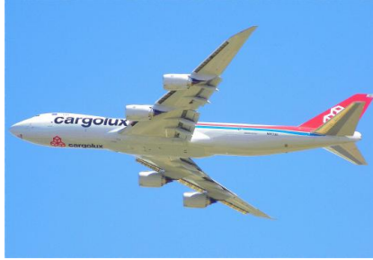
Figure 1.3: Highly flexible wing of the Boeing 747-8, prone to flutter (source of picture: [131])
