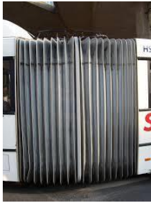
Figure 6.3: Corrugated bellow in an articulated bus (source of picture: [89])
