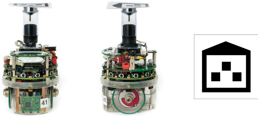
Fig. 1 Front and side view of an e-puck robot and a tag used to localize the robot via a ceiling-mounted camera
