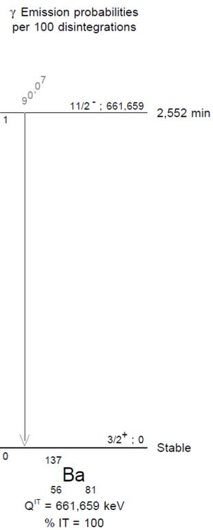
(A.6.17-1)  $^{137\text{m}}\text{Ba}$  decay scheme,  $T_{1/2} = 2.55 \text{ m}$
