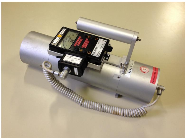
Figure 3.5: AUTOMESS 6150AD6/H with the scintillation probe AUTOMESS 6150AD-b/H and the Bluetooth adapter AUTOMESS BlueCOM-Adapter 910.1.
