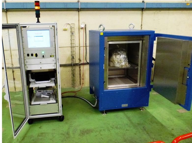
Figure 3.2: RADOS RTM 661/440 Inc installed in the CERN ISR (Intersecting Storage Rings) clearance facility of the Radioactive Waste Section of the CERN Radiation Protection Group.
