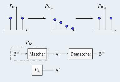
Figure 1 : Matching a data block  $B^m = B_1 \dots B_m$  to output symbols  $\tilde{A}^n = \tilde{A}_1 \dots \tilde{A}_n$  and reconstructing the original sequence at the dematcher. The rate is  $\frac{m}{n} \left[ \frac{\text{bits}}{\text{output symbol}} \right]$ . The matcher can be interpreted as emulating a discrete memoryless source  $P_A$ .
