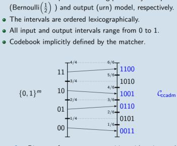
Figure 2 : Diagram of a constant composition arithmetic encoder with  $P_{\bar{A}}(0) = P_{\bar{A}}(1) = 0.5, m = 2 \text{ and } n = 4.$
