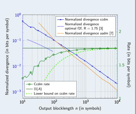
Figure 3 : Normalized divergence and rate of ccdm over output blocklength.  $P_A = (0.0722; 0.1654; 0.3209; 0.4415).$
