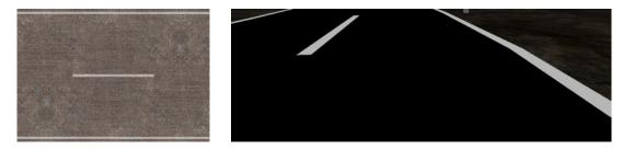
**Figure 5.12:** Examples of road surface textures with high (left image) and low (right image) contrast. The image on the right is an example of the previous driving simulator of the Institute for Human-Machine-Communication. In the new version speed perception is improved to generate more realistic experimental results.
