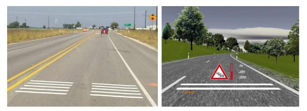
**Figure 3.22:** Picture of real rumble strips for speed reduction (left) and the implementation in the HUD (right). Several sets of rumble strips were installed upstream a construction site with small but statistically significant speed reductions (see [Mil+05]). Every time a virtual strip passes "under" the ego vehicle a rumble sound is produced by the subwoofer in the driver seat creating vibrations for haptic feedback (scene and HUD content digitally mixed).
