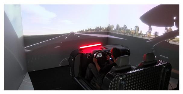
**Figure 6.31:** View of the driving simulator consisting of a real car cockpit with the ISPA LED system and the CAVE for environment projection
