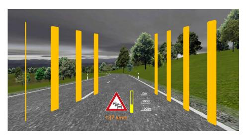
**Figure 3.24:** Picture of the vertical bars produced by the contact analogue Head-Up Display. The bars can be used to alter the speed perception and also the perceived width of the road causing a speed adaption (scene and HUD content digitally mixed).
