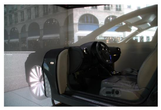
**Figure 5.8:** Combination of real and virtual elements of the driving simulator mockup. All directly reachable parts for the driving part are represented by a physical mockup while elements like front wheels, ceiling etc. are added virtually.
