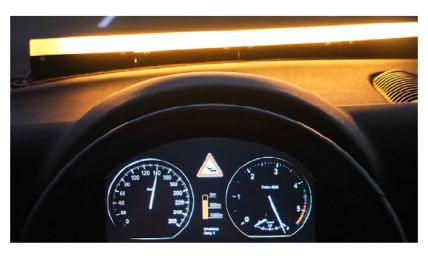
**Figure 6.32:** ISPA output devices: RGB-LED array on top of the dashboard for encoding distance and proposed deceleration strategy, icon graphics in the instrument cluster depicting the obstacle type and the distance
