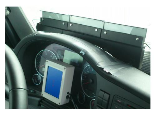
**Figure 4.5:** Picture of the LED modules and the instrument cluster display. The auxiliary display is small enough to maintain a free sight on the built-in instrument gauges.
