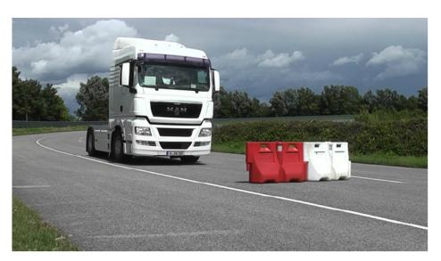
Figure 4.1: Barrier representing an obstacle on the ego lane
