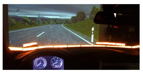
**Figure 3.37:** Driver view of the two LED arrangements on the engine hood. For demonstration purposes all LEDs of both HMI variants are illuminated.
