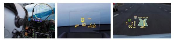
**Figure 3.10:** Implementations of Head-Up displays. First applications were military aircraft (left), later the technology was adopted for cars (center and right picture).
