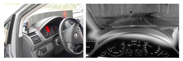
**Figure 3.30:** LED modules for augmenting a Night Vision system. Left: The system displays a simple icon using the LED matrix in the actual line of sight between the driver's head and the obstacle recognized by the NiVi system (image from [Wei+09]). Right: LED line activating a group of LEDs in the line of sight towards the obstacle (image from [Mah+07]).
