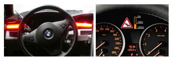
**Figure 3.32:** First LED prototype in combination with instrument cluster visualization. The instrument cluster shows the Iconic HMI, the LED modules are installed left and right of the steering wheel.
