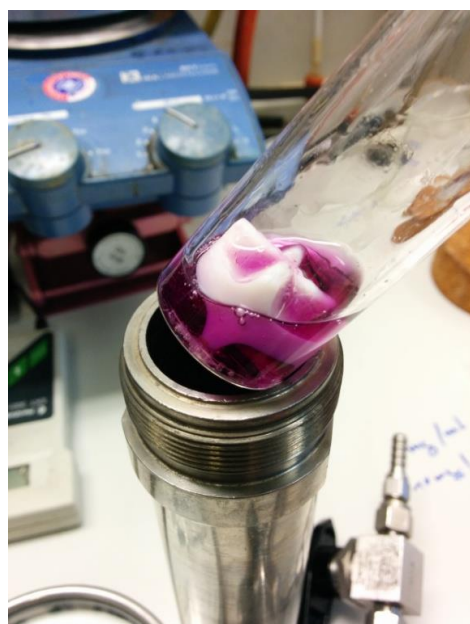
Figure S15. Copolymerization experiment with catalyst 3-MeOH in an autoclave immediately after CO 2 release and opening of the autoclave (3-MeOH/CHO = 1:500, cat/DMAP = 1, 18 h, 80 °C, 50 bar).
