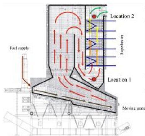
Figure 1: Schematic illustration of the wood fired power plant Schkölen with measurement locations
