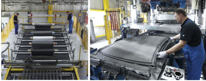
Figure 6.19: Manufacturing of a BMW M3 CFRP rooftop: automated stacking of the single UD-ply (left) and preforming of the stack (right) [93]
