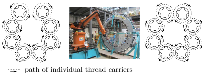
Figure 1.6: Braided fabrics: schematics of a band-shaped fabric (left), radial braiding machine (center), schematics of a tube-shaped fabric (right) [source: Figure 8.4 in CHERIF ET AL. [33], Figure 4.4.1 - 4.4.2 in FLEMMING ET AL. [42], [43]]
